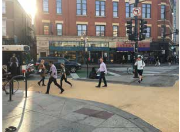
Slip lane closure at the Milwaukee Avenue, North Avenue, and Damen Avenue intersection improves safety and creates new pedestrian space.
